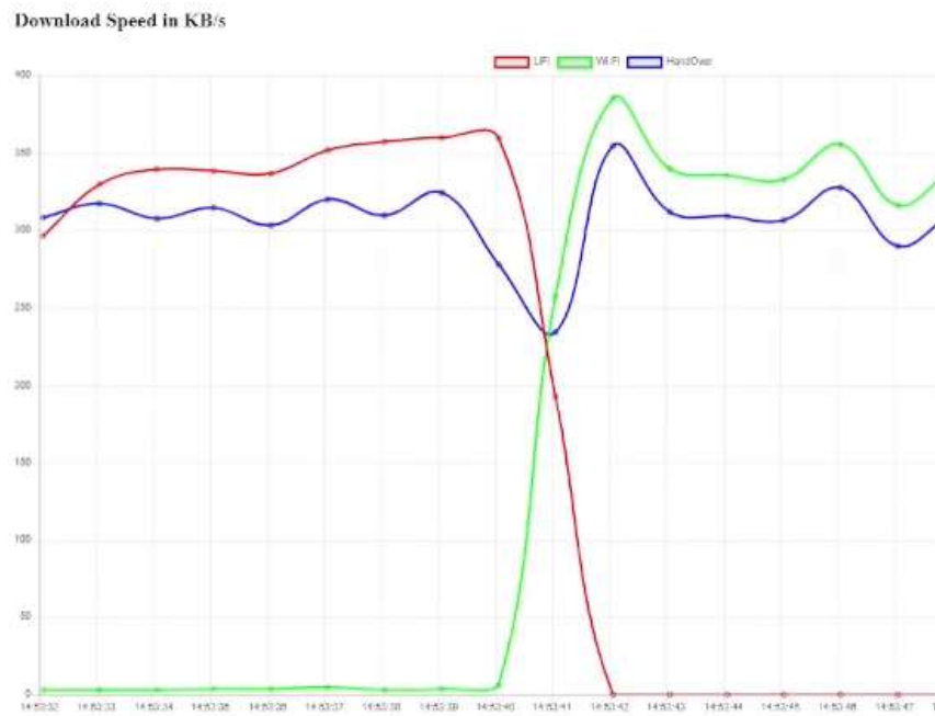
Figure 4. Handover from Li-Fi to Wi-Fi: Download Speed in KB/s during a MS teams call
