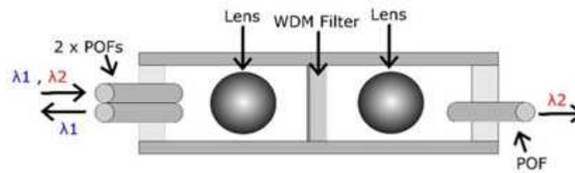
Figure 15 MUX/DMX structure.
