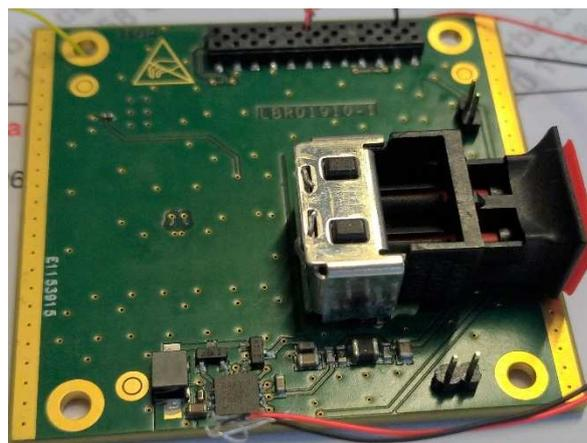
Figure 14 Red color POF transceiver composed by a red RC-LED, photodiode and electronics on a PCB.
