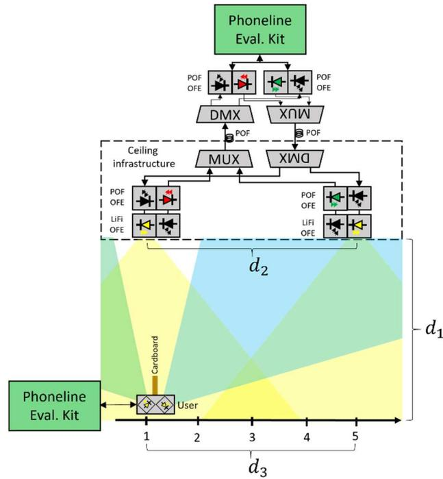
Figure 10 Illustration of the WDM over POF fronthaul used to feed signals to a 2x2 MIMO D-MIMO LiFi communication system.
