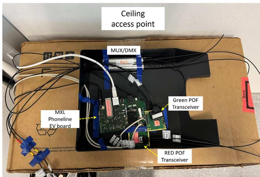
Figure 17 Ceiling access point: MXL Evaluation Kit connected to two POF transceivers and WDM-POF fronthaul components.
