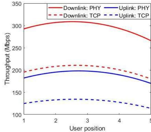
Figure 19 Measured (downlink and uplink) throughput performance WDM-over-POF fronthaul feeding a 2x2 D-MIMO LiFi link.
