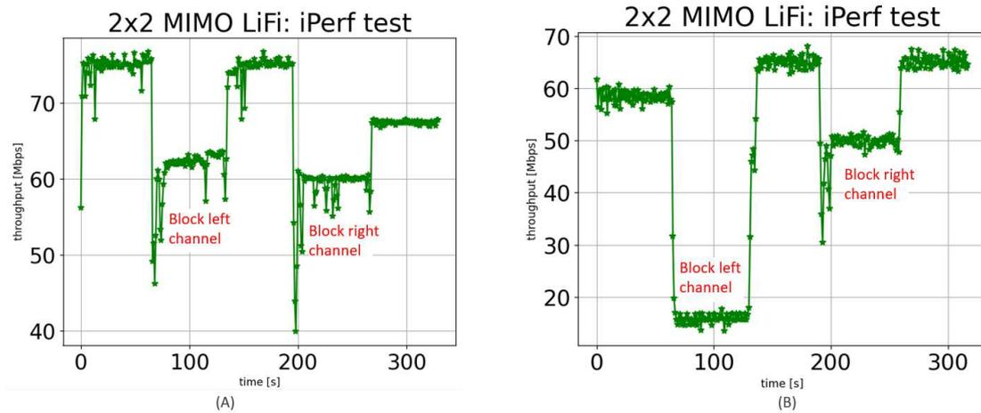
Figure 8: Impact of partial line-of-sight blockage when mobile device was placed under ceiling OFE5: (A) downlink, (B) uplink
