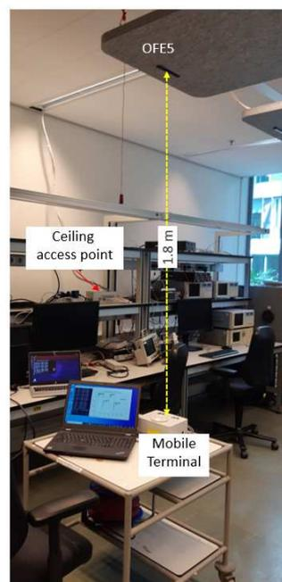
Figure 3: LiFi-MIMO demonstrator test setup. Two laptops are used as data source and sink to evaluate the link performance using iPerf and Spirit Configuration tools.
