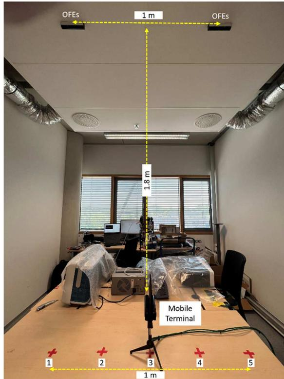
Figure 11 Office demonstrator: WDM fronthaul feeding 2x2 D-MIMO LiFi.
