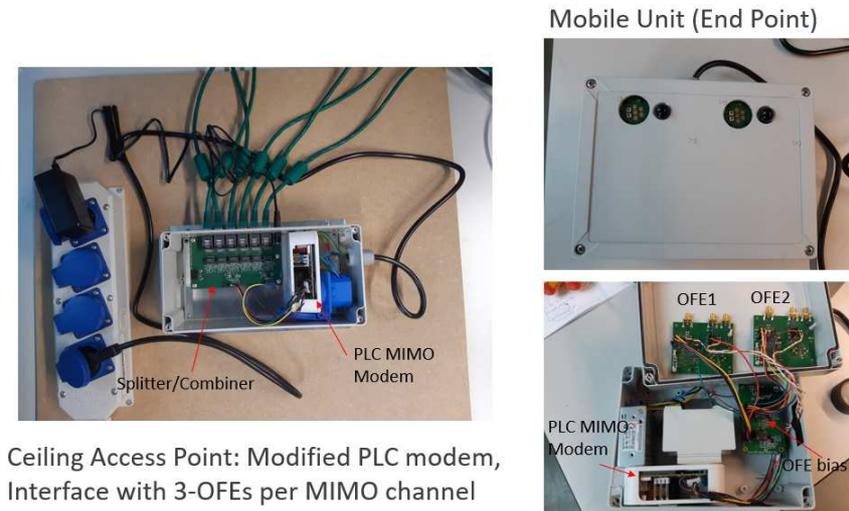
Figure 4: Office demonstrator components.
