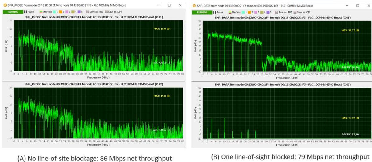
Figure 7: Signal-to-noise ratio (SNR) plot of downlink without and with line-of-site blockage and respective net throughput.
