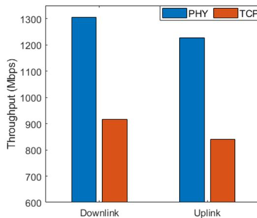
Figure 18 Raw and iPerf measured throughput for the WDM over POF link, considering 10 m of fronthaul length.
