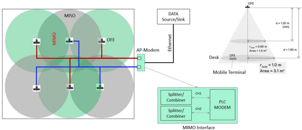
Figure 1: Architecture of office demonstrator.
