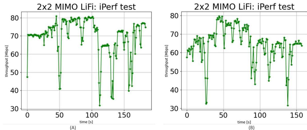
Figure 9: Impact of mobility on throughput: (A) downlink. (B) uplink.
