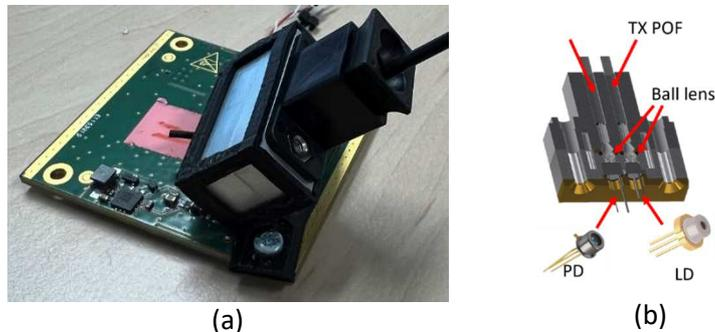
Figure 13 (a) Green color POF transceiver composed by a green laser diode, a photodiode and electronics on a PCB. (b) POF transceiver package designed at TU/e.
