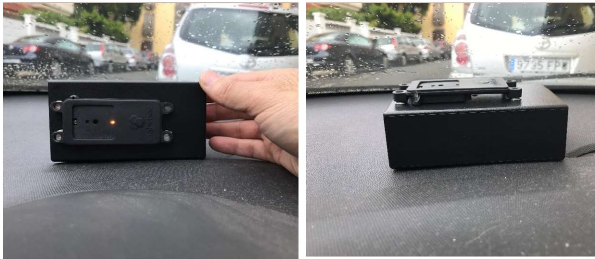
Figure 11 Control access system with VLC in rent a car usage concept. Applied to an electrical car from PSA in Vigo (Spain)
