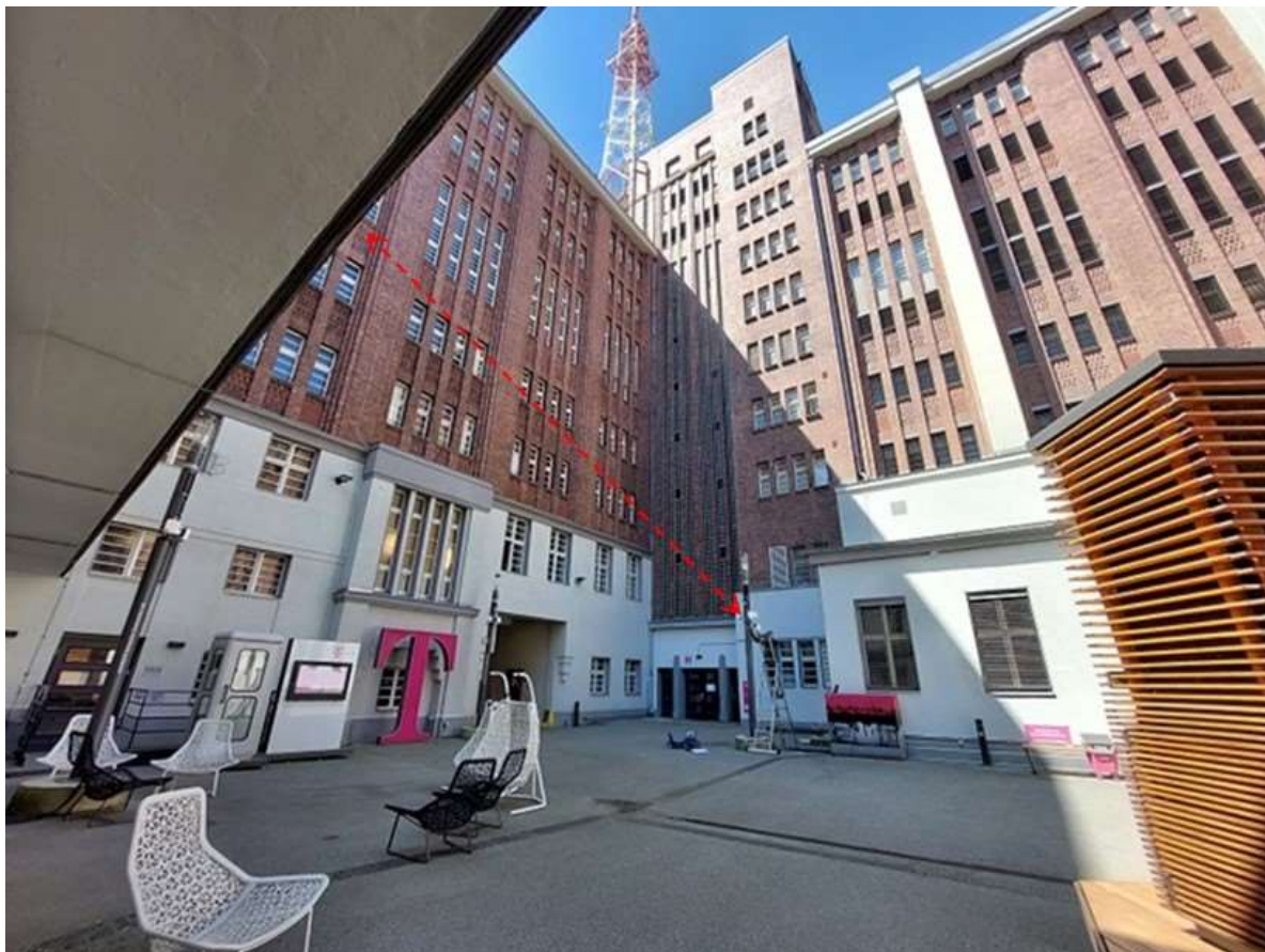
Figure 5 Outdoor test environment with PtP OWC link between distribution node (DN) and client node (CN)
