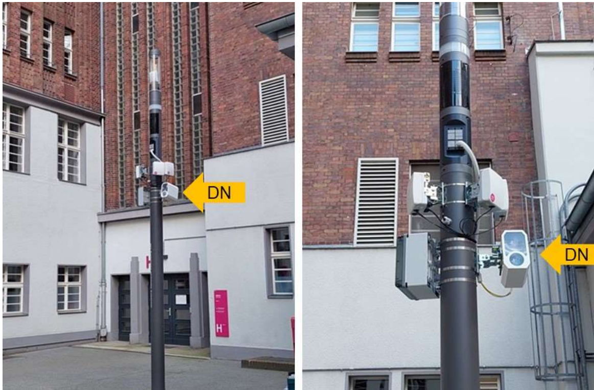
Figure 3 Distribution node (DN) mounted at the lamp pole in the outdoor test environment
